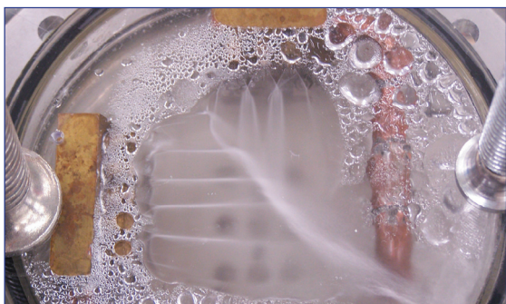
Spray Impingement cooling test for prototype high volume optical device development
