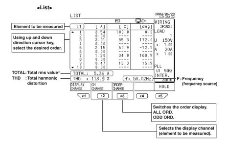
TOTAL: Total rms value\*: Total rms values are displayed if the elements to be measured are voltage (I) and current (I); total power values are displayed if the element to be measured is power (P).
