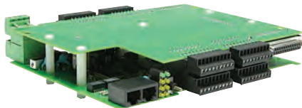
Interface to isolated 8B analog output modules.
