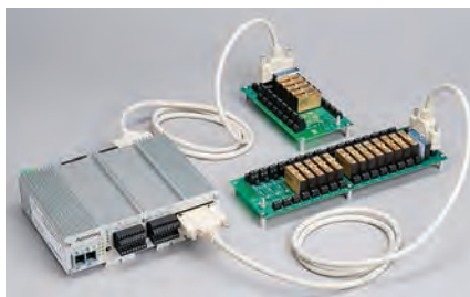
Interface to 8B signal conditioning modules.
