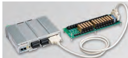
Interface to isolated 8B analog output modules.
