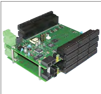
ESA-OMK open board stacking kit. One kit supplies standoffs to stack two units.
