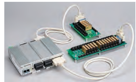
8Bs also connect to EtherStax analog I/O modules (ES2151, ES2152, ES2153, ES2162, ES2172 models)
