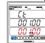
The screen changes to the one for setting the parameter **CL**. The lower display shows the current value and the decimal point blinks.
