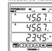
The PR300 shows the Startup screen for about 5 seconds, then the Measured Value screen appears.
