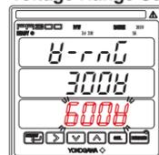
Pressing **SET/ENT** once causes all digits of the setpoint to start blinking. Pressing **SET/ENT** once again confirms the setpoint and returns to the Voltage Range screen.
