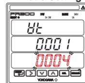
Pressing **SET/ENT** once causes all digits of the setpoint to start blinking. Pressing **SET/ENT** once again confirms the setpoint and returns to the VT Ratio screen.
