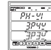
Pressing **SET/ENT** once causes all digits of the setpoint to start blinking. Pressing **SET/ENT** once again confirms the setpoint and returns to the Phase and Wire System screen.
