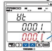
The screen changes to the one for setting the parameter **VL** and the alterable digit blinks.
