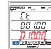
Pressing **SET/ENT** once causes all digits of the setpoint to start blinking. Pressing **SET/ENT** once again confirms the setpoint and returns to the CT Ratio screen.
