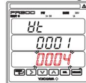
Pressing **SET/ENT** once causes all digits of the setpoint to start blinking. Pressing **SET/ENT** once again confirms the setpoint and returns to the VT Ratio screen.
