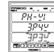
Pressing **SET/ENT** once causes all digits of the setpoint to start blinking. Pressing **SET/ENT** once again confirms the setpoint and returns to the Phase and Wire System screen.
