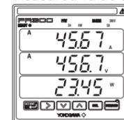
The PR300 shows the station number for about 5 seconds, then the Measured Value screen \* appears.
