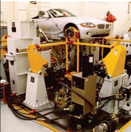
Schedule demands and cost control require new paradigms to reduce the cost of test, and reduce the time needed for test setup. Typical measurements include Strain, Load, Pressure, and displacement. Channel counts continue to increase to provide the Analyst a better understanding of the structure to help make better design changes or improvements.
