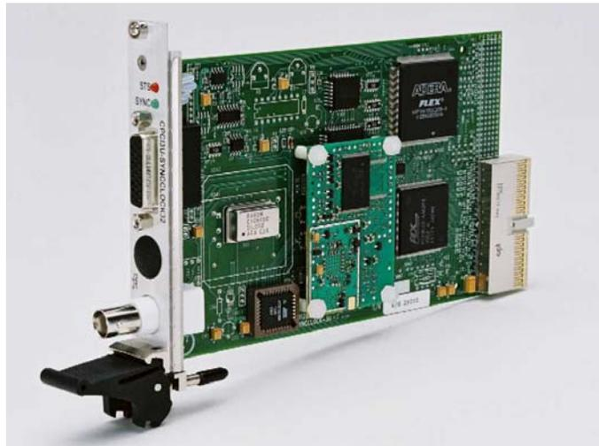
The CPCI-SyncClock32 from Brandywine Communications provides precision time with zero latency to the host computer over the CPCI bus in the 3u form factor. An on-board microprocessor automatically synchronizes the clock to reference signal inputs. The reference signal inputs can be 1 PPS, IRIG or NASA time codes and optionally, GPS or Have Quick. The clock can free run and be set by commands from the host over the CPCI bus.
