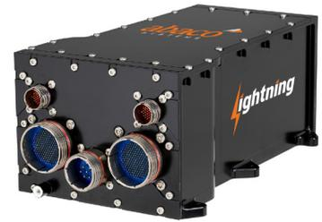
Qualification takes the form of testing for temperature, temperature shock, altitude, humidity, shock/vibration, EMI, sand/dust, salt spray, water ingress and flammability to standards such as MIL-STD-810G method 514.7, 516.6, DO-160G Sections 4-21, 25 and MIL-STD-561G.
