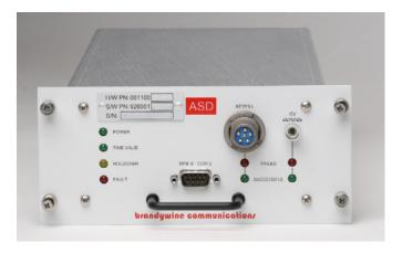
The PTS-SAASM is a state of the art frequency instrument offering a wide range of features and time and frequency outputs accurate to < 40ns <sub>rms</sub> to UTC (USNO) and  $1x10^{-12}$  respectively.
