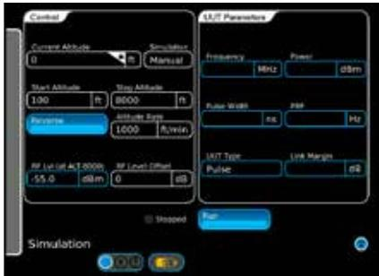
Simulated static altitude may be set by the user and manually incremented or decremented.
