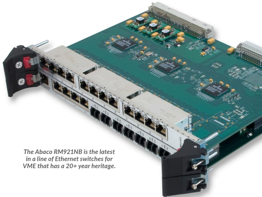
*The Abaco RM921NB is the latest in a line of Ethernet switches for VME that has a 20+ year heritage.*
