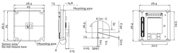
Sensor and electronic components are schematics and vary between models.
