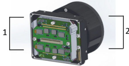
Figure 9: Front assembly overview: sensor unit and lens mount
