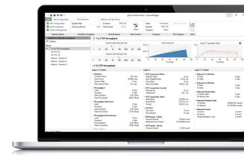
VulcanAppMix (VAM) is a library of application traffic and protocols in pcap format. VAM makes it easy to set up large-scale realistic traffic from various applications, using pre-defined and customizable mix templates. Up to 200 pre-defined application scenarios can be played simultaneously, each covering a one-client-to-multiple-servers communications scenario that can be scaled up to millions of connections with real-world traffic.
