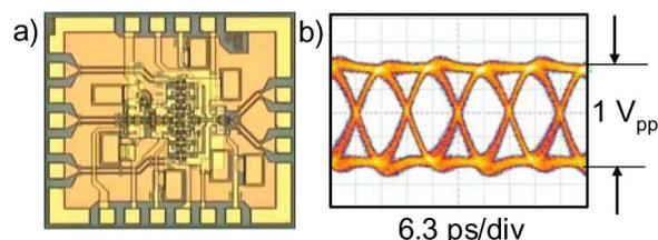
Fig. 2. (a) Microphotograph of the 2:1 InP HBT multiplexer; (b) electrical output eye diagram at 80 Gb/s for a PRBS  $2^{15} - 1$ .
