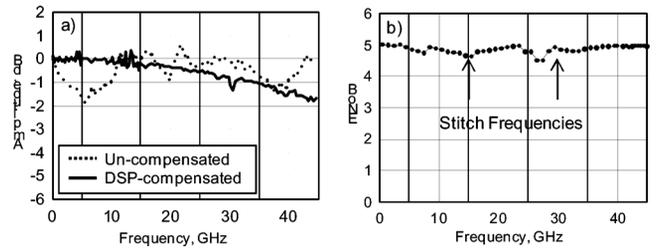
Fig. 4. (a) Amplitude response of the 45-GHz acquisition system before and after DBI processing. (b) ENoB measurement to 45 GHz.
