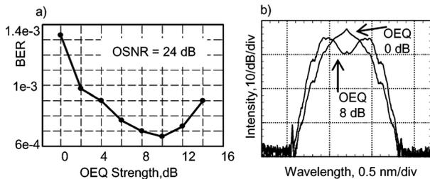
Fig. 6. (a) Optimization of OEQ at 24-dB OSNR. (b) Optical spectra for 8- and 0-dB OEQ, corresponding to BER and constellations of Fig. 5.
