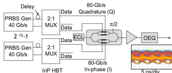
Fig. 1. 80-Gbaud (160-Gb/s) single-polarization QPSK transmitter. Inset: Optical QPSK eye diagram measured at  $2^{15} - 1$  PRBS length.
