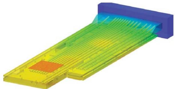
$$k_{\text{eff}} = \frac{25 \text{ W} \times 0.056 \text{ m}}{(3.004 \times 10^{-6}) \times 2 \text{ K}} = 233,000 \frac{\text{W}}{\text{m K}}$$
