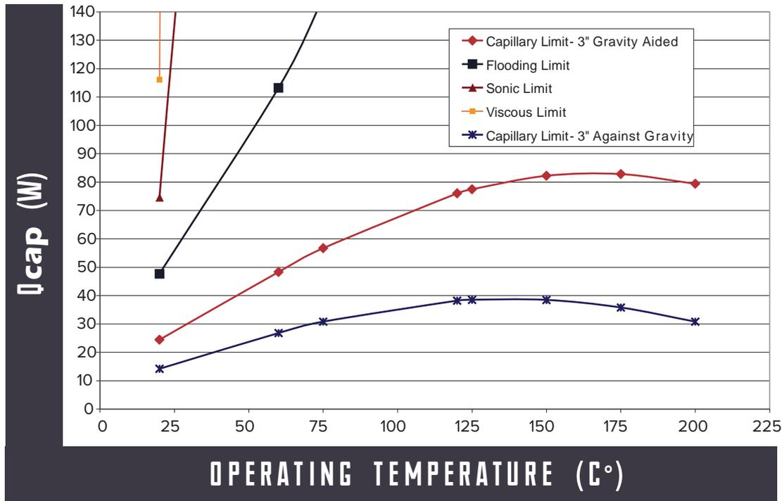
This graph shows the various heat pipe limitations for a typical copper/water heat pipe. These limitations are a function of the operating temperature, due to the change in the fluid properties as a function of temperature. It is important to ensure that the appropriate performance limit curve adequately covers the performance requirement for the entire specified temperature range.
