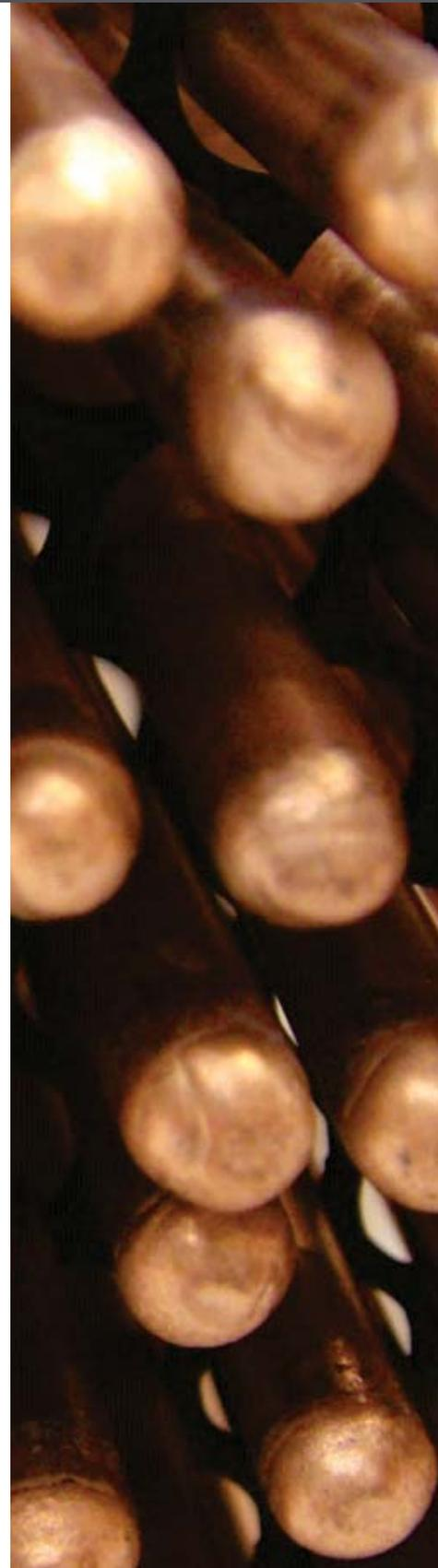
Copper/water heat pipes are used in a wide range of applications, most notably in electronics cooling. Water is an ideal fluid to operate and cool components nearing the maximum case temperature of electronics (70 to 100 C). Additionally, because water has favorable surface tension properties, heat pipes can be designed to operate in any orientation.
