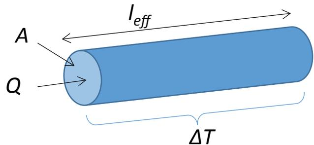
$$l_{\text{eff}} = \frac{l_{\text{evap}} + l_{\text{cond}}}{2} + l_{\text{ad}} = 2.21 \text{ in} = 0.056 \text{ m}$$
