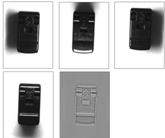
Figure 1 - A black plastic clip is inspected using four LED bar lights, a light controller, and the Matrox Image Library processing software. Photos courtesy of Matrox Imaging.
