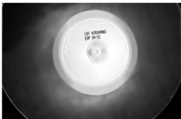
Figure 7B - Final processed image of the bottom of the glossy vitamin bottle
