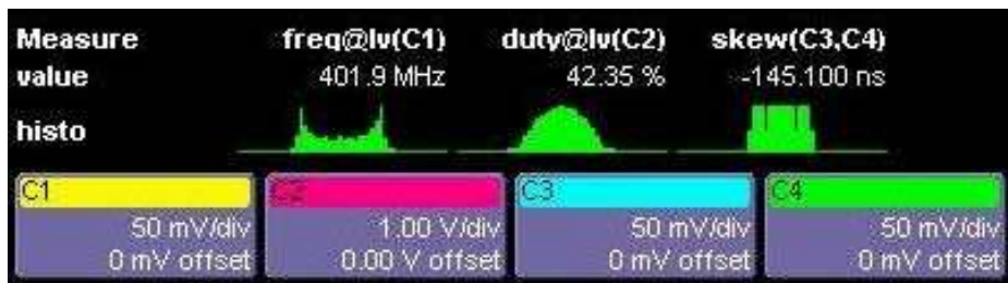
Figure 1: Histicons (histogram icons) showing frequency modulation, noisy duty cycle and a flat distribution of timing skew.
