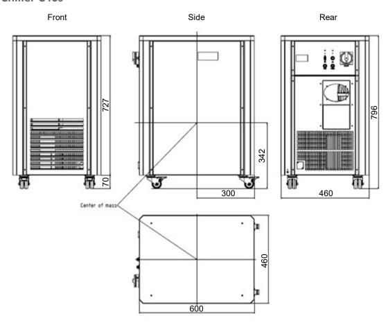
C40s Thermal System: -40°C to +300°C
