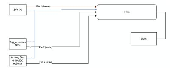
Analog input is pulled HIGH internally and can float if unused or tied to +24VDC. A trigger is required to enable the output. If using continuous, the trigger may be tied directly to +24VDC.
