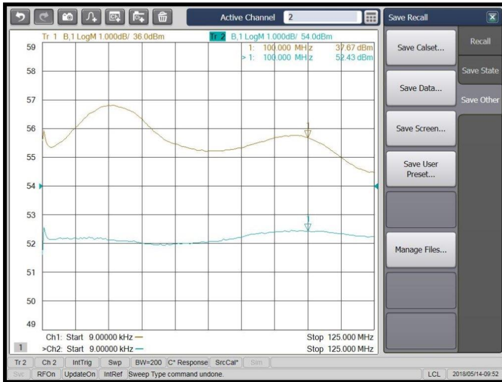
Figure 4-1. Typical Response at -20 dBm Input and 0 dBm Input
