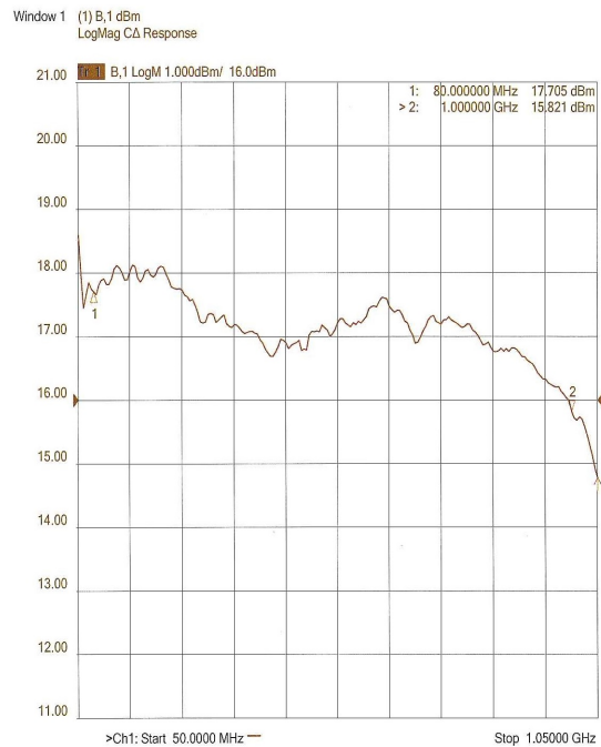
Figure 4-3. Typical Response: Input A3–Front Panel RF Output
