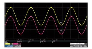
Output amplitude into a high impedance load can be as high 20 Vpp at frequencies up to 10 MHz, and 10 Vpp for frequencies greater than 20 MHz.
