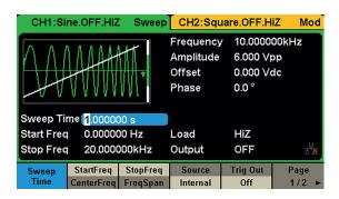
Sweep mode supports 'Linear' and 'Log' sweep, with 'Up' and 'Down' direction, and Sweep source can be configured as 'Internal', 'External' or 'Manual'.
