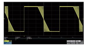
The rise/fall times can be set independently to a minimum of 16.8 ns at any frequency and to a maximum of 22.4s.
