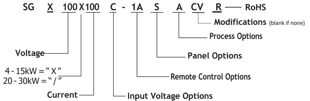
(For units with greater than 3 digits, Voltage/Current is represented in numeric format, e.g., above "100" represents 100A. For units at 1000 and above, the voltage is represented by the format "XKX", e.g, 1K2 = 1200V and 1K0 = 1000V)
