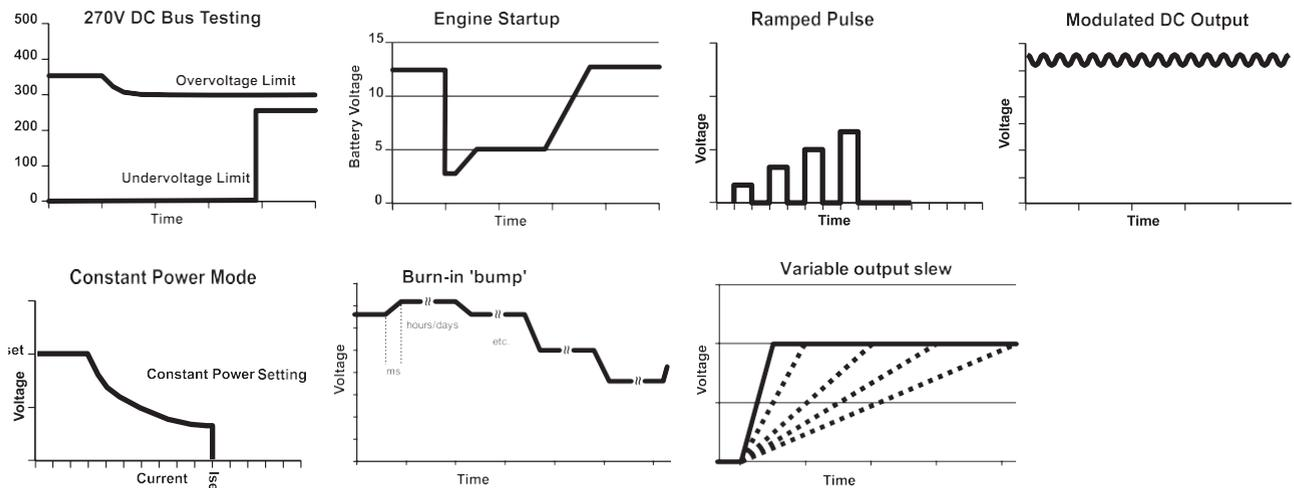
SGX model provides constant power mode allowing independent setting of the max voltage, current and power
