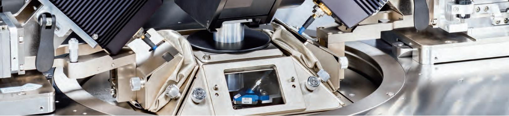
*"Only the **Autonomous RF Measurement Assistant**, a combination of programmable positioners, a precise digital microscopy system and advanced pattern recognition algorithms, enables fully autonomous, hands-free calibrations and measurements of RF devices over multiple temperatures."*
