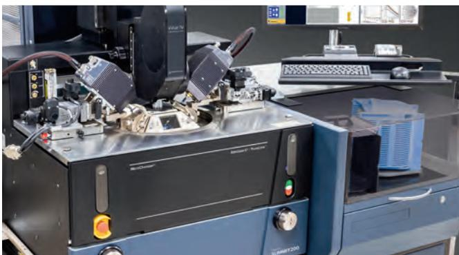
With the optional loader that is available for the SUMMIT200 and CM300xi, the system combines fully-automated wafer test with highest accuracy and flexibility. The loader can handle up to fifty wafers provided in SEMI-standard wafer cassettes.
