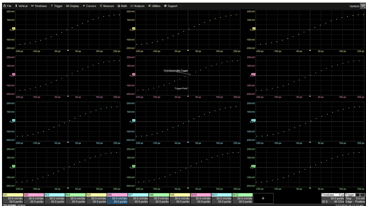
Figure 2 The horizontal offset, time delay between the trigger and the next sample, is uniformly distributed over the sampling period; multiple acquisitions show this variation.
