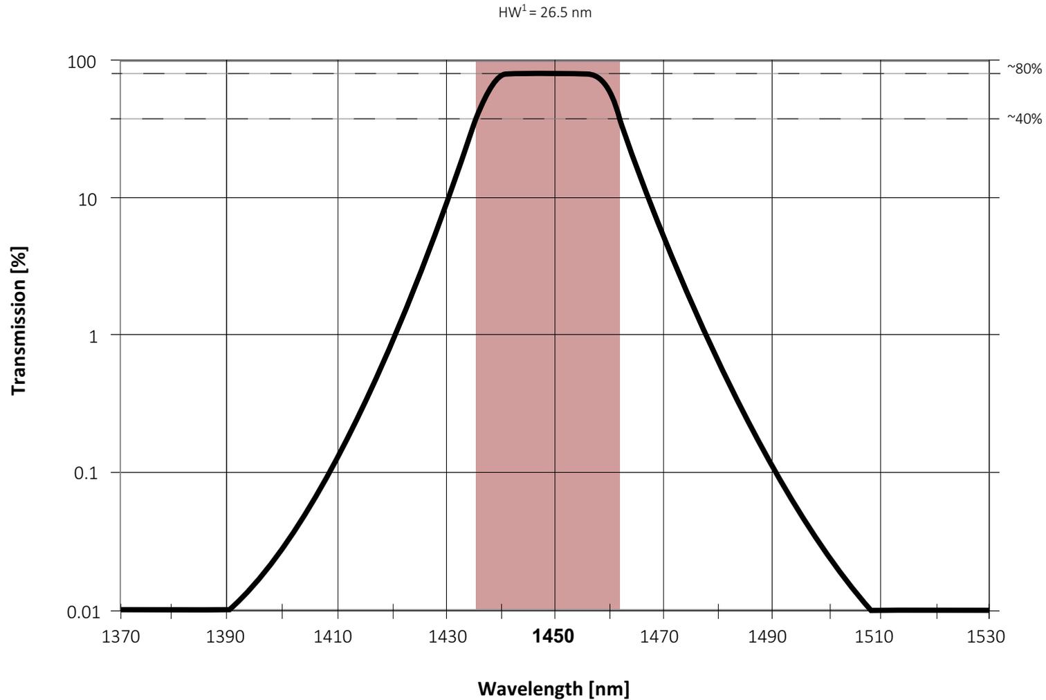
Figure 5: Spectral transmission of IRBP 1450 nm (IR bandpass filter, exemplary curve)
