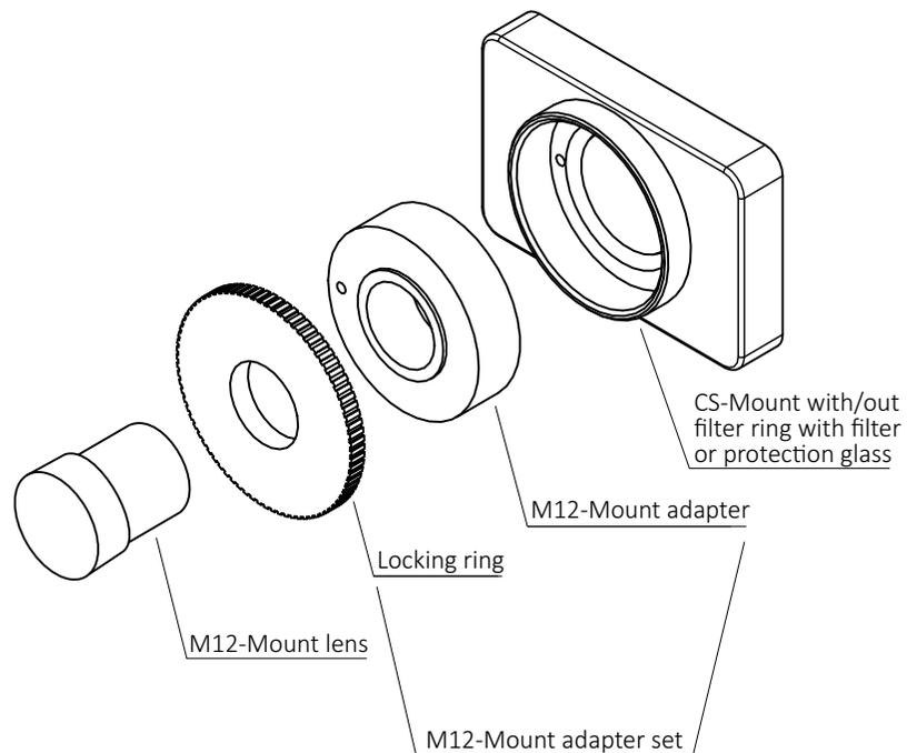
Figure 1: M12-Mount lens adapted to CS-Mount with the M12-Mount adapter set
