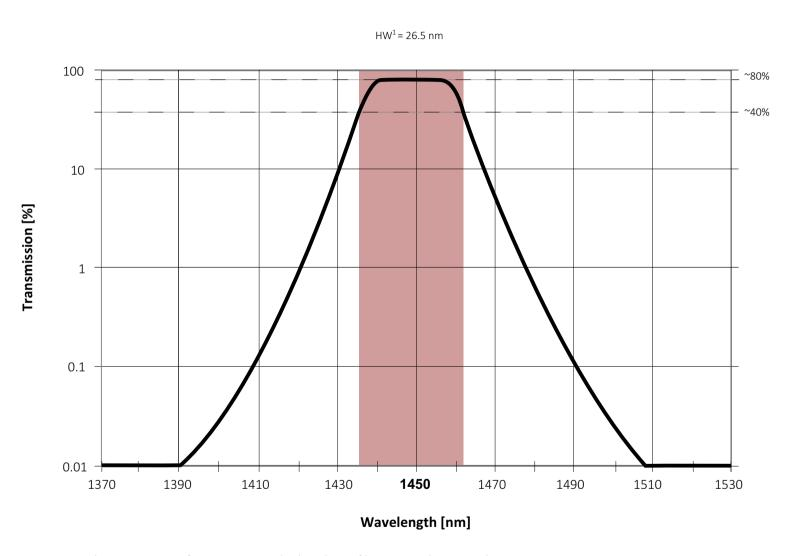
Figure 5: Spectral transmission of IRBP 1450 nm (IR bandpass filter, exemplary curve)
