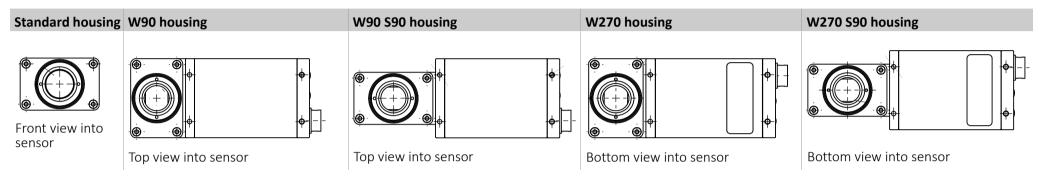
Figure 2: Sensor position of standard housing and angled head options.
