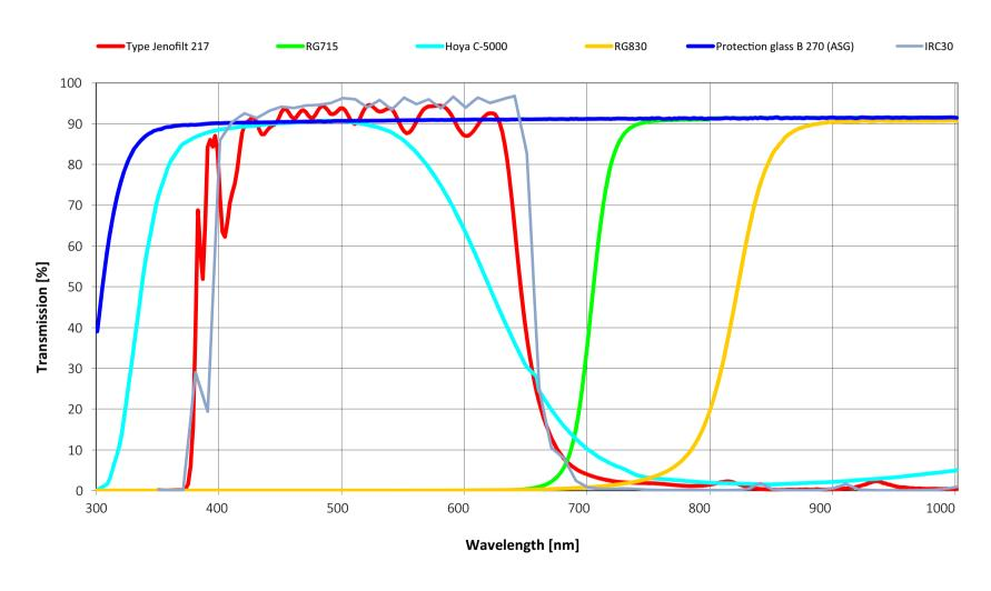
Figure 4: Spectral transmission of filters 300 to 1000 nm (exemplary curves)
