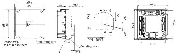
Sensor and electronic components are schematics and vary between models.
