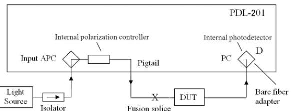
Figure 7 Production floor setup to measure an unconnectorized, pigtailed DUT using only fusion splice and bare fiber adapter to connect to the PDL-201.
