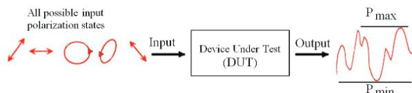
Figure 1 Illustration of PDL definition
