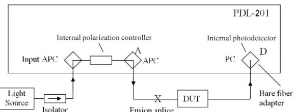
Figure 6 Production floor setup to measure an unconnectorized, pigtailed DUT using fusion splice to a free pigtail and bare fiber adapter to connect to the PDL-201.
