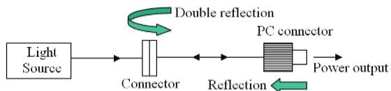
Figure 2 Illustration of double reflection
