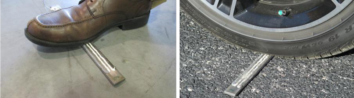
Figure 4: Fiber sensor with protective coating applied, being stepped on and driven across, with no degradation of data quality.
