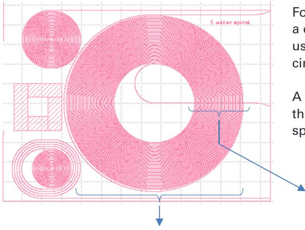
For example, the Optoelectronics Research Group at UCSB fabricated a one meter spiral delay line on a silicon platform. The OBR 4600 was used to measure the distributed loss inside the photonic integrated circuit (PIC), which measured only 1 cm<sup>2</sup> in size.
