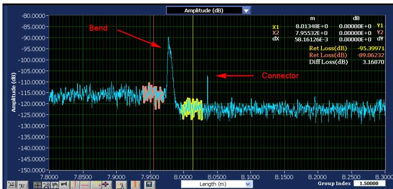
Use convenient cursor tools to measure and examine scatter level and reflection events to measure RL and IL for closely spaced events.
