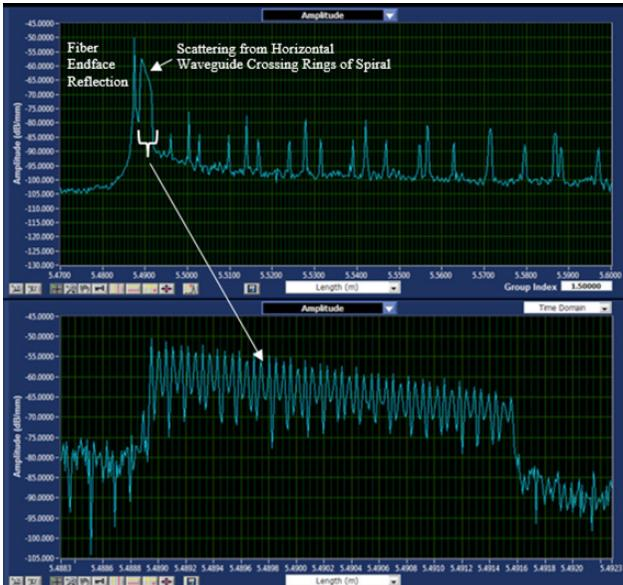
The high spatial resolution of the OBR 4600 is used to illuminate a reflective event near the entry point of the spiral delay line. The detail in the lower plot reveals that the broad reflective event at the beginning of the trace is in fact a series of 50 individual reflections in the space of 2.5 mm correlating to the input waveguide leg crossing the arms of the spiral path.
