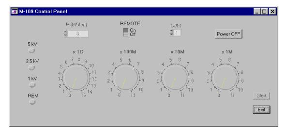
The light of indicating elements on the left-hand part of the screen is corresponding to LED diodes on the instrument panel. Rotary buttons on the control panel are displayed like "enable". They are only indicators of the real switches setup position on the front panel of the instrument now.
