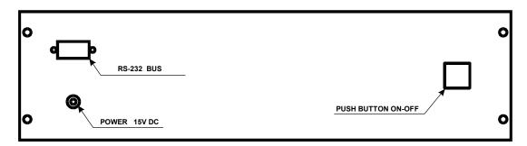
On the rear panel is the ON/OFF button for switching the decade on and off, supplying connector and a connector for connecting RS-232.
