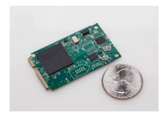
The exact time-of-occurrence of random external events may be captured by using the Event Time input. When the event input is sensed the current time is saved in a buffer for later interrogation by the host. The resolution of the time tag is 100 nanoseconds.
