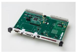
Brandywine Communications' VME635091-SYNCCLOCK time and frequency processor module provides precision time and frequency reference to the host computer and peripheral data acquisition systems. Time is acquired from time code signals, typically IRIG B. Time is displayed on the front panel (hours, minutes, seconds) via LED digits.
