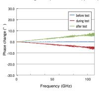
\*The cable was wrapped 90° around  $\phi$  30mm mandrel.
