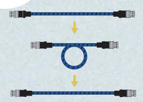
The cable was wrapped  $360^{\circ}$  around  $\phi 60$ mm mandrel. \*Guaranteed value within ±5.7°at 26.5GHz (In shipping value)
