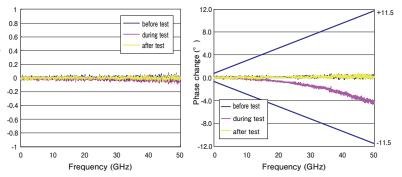
\*Guaranteed value within ±11.5° at 50 GHz (In shipping value). \*The cable was wrapped 360° around  $\phi$  60mm mandrel.
