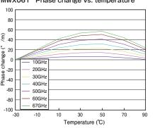
The cable was measured in chamber every 20 ℃ from -30 to 90 °C, 1 hour after the temperature changed. Figure shows the excellent phase stability over the temperature changes.
