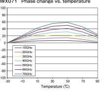
The cable was measured in chamber every 20 ℃ from -30 to 90 °C, 1 hour after the temperature changed. Figure shows the excellent phase stability over the temperature changes.
