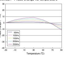
The cable was measured in chamber every 20 °C from -30 to 90 °C, 1 hour after the temperature changed. Figure shows the excellent phase stability over the
