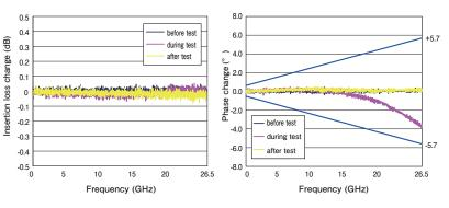
\*Guaranteed value within ±5.7° at 26.5 GHz (In shipping value) \*The cable was wrapped 360° around  $\phi$  60mm mandrel.
