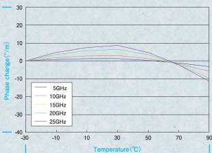
The cable was measured in chamber every 20 °C from -30 to 90 °C, 1 hour after the temperature changed.
