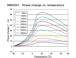
\*The cable was measured in chamber every 20 °C from -40 to 90 °C, 1 hour after the temperature changed.
