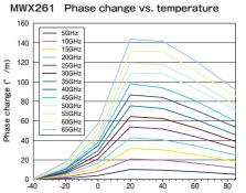
\*The cable was measured in chamber every 20 °C from -40 to 90  $^{\circ}\!\text{C},$  1 hour after the temperature changed.
