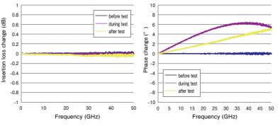
\*The cable was wrapped 360° around \$\phi 40mm mandrel.
