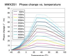
\*The cable was measured in chamber every 20 °C from -40 to 90 °C, 1 hour after the temperature changed.
