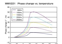
\*The cable was measured in chamber every 20 °C from -40 to 90 °C, 1 hour after the temperature changed.
