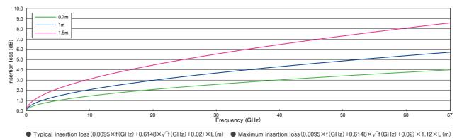
\*The cable was wrapped 360° around \$\phi 40mm mandrel.
