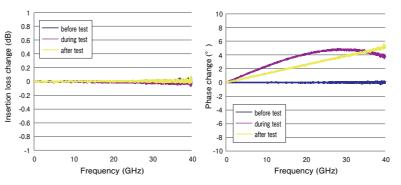
\*The cable was wrapped 360° around \$\phi 40mm mandrel.
