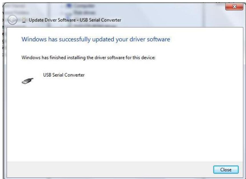
5. When the installation is finished, a "software successfully updated" message will appear. This completes the first part of the installation, during which the USB to serial converter is installed. The second part consists of the installation of the serial port driver.
