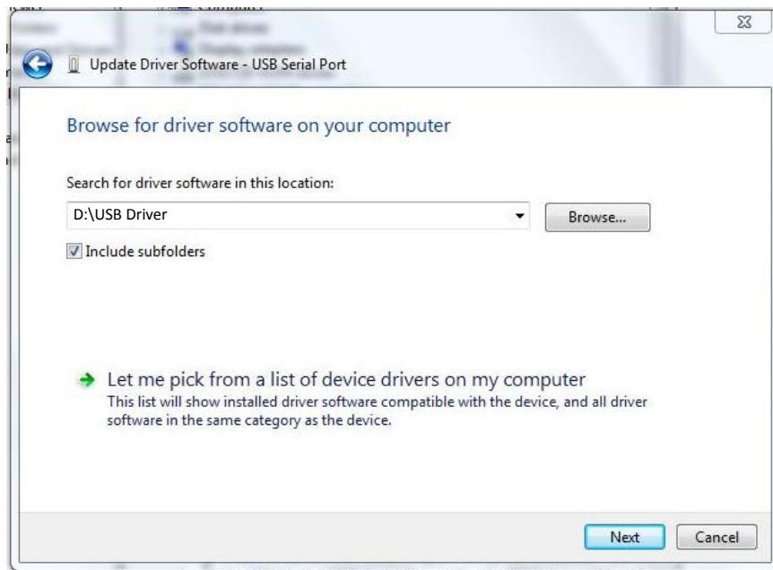
3. Make sure that the software cd is inserted. Click "Browse", navigate to the cd drive, and select the "USB Driver" folder. Make sure the "include subfolders" box is checked. Click "Next".
