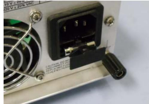
**Figure 6 Fuse compartment**
