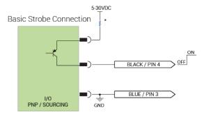
\*External resistors may not be needed Check documentation on I/O for recommendations and voltage limits Analog Dimming
