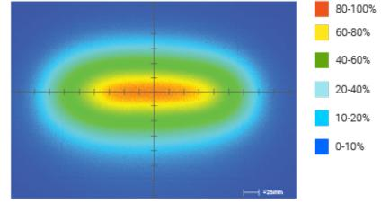
Optical measurement taken using AL-S025300M-WHI @ 300 mm
