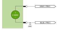
Analog dimming works in both strobe and continuous
