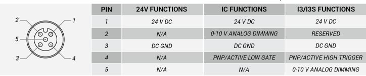
The functions listed above are only applicable when this product is configured with built-in 24V, IC, I3, or I3S control, with an A-coded 5-position Male M12 connector.
