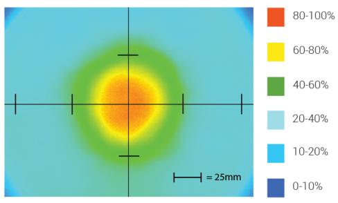
Optical measurement taken using DF241-62525I3 @ 12.5 mm
