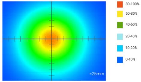
Optical measurement taken using RL-S052120M-WHI @ 300 mm
