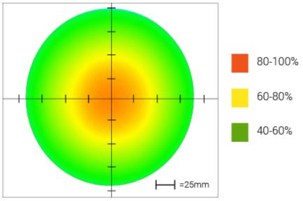
Optical measurement taken using RL127-WHIIC @ 200 mm
