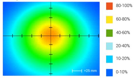
Optical measurement taken using RL1424-660100LC2 @ 200 mm
