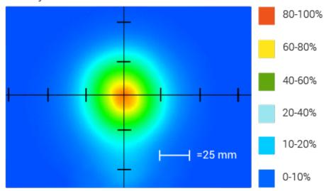
Optical measurement taken using RL2115-WHII3 @ 9.5 mm
