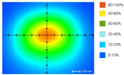
Optical measurement taken using SL-S100150M-WHI @ 300 mm
