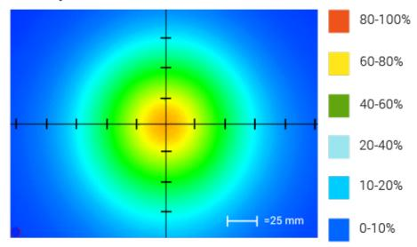
Optical measurement taken using SL164-WHIIC Rev. A @ 300 mm
