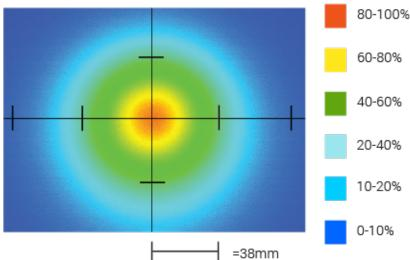
Optical measurement taken using SL223-WHIIC @ 75mm
