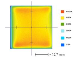
Optical measurement taken using BT050050-WHII3
