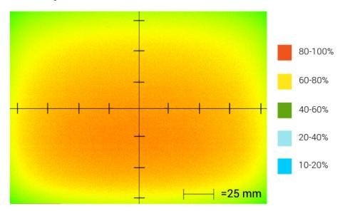
Optical measurement taken using DL067A12-WHIIC Rev. A @ 25mm
