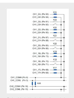
Embedded virtual schematic control simplifies setup and debugging; allows all relays to be engaged independent of application software and device drivers.
